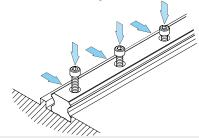
5 Tighten the mounting bolts with a torque wrench to the specified torque.
