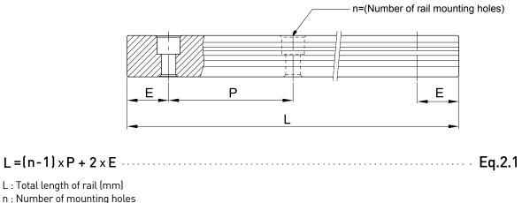
P : Distance between any two holes (mm)
