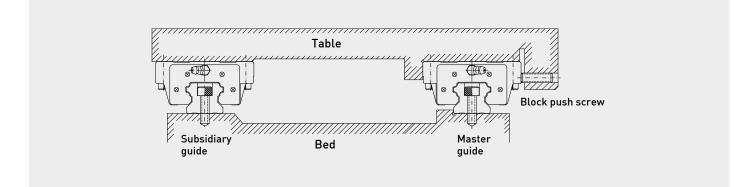
(1) Installation of the rail on the subsidiary guide side
