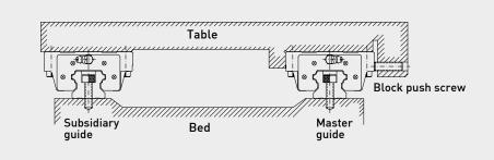
(1) Installation of the rail on the master guide side
